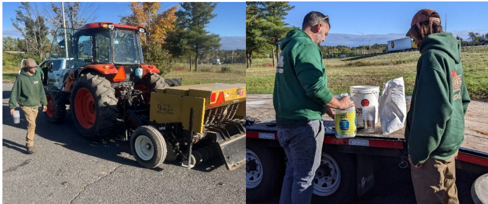
Figure 5. October 16, 2023. Fall seeding of CT site: Truax drill (left); mixing seed with clay cat litter carrier (left).
