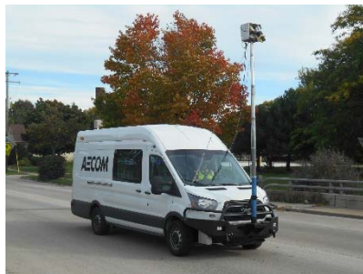
Figure 4 - Van Equipped with IR Sensor
