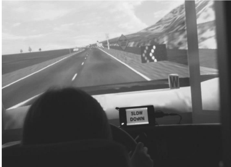
Figure 12 Visual In-Vehicle Display Installed in the Simulator [36]
