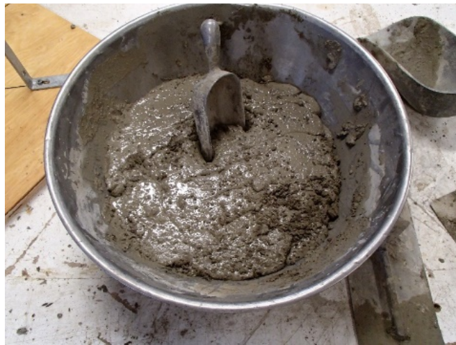
Figure 4-4: Concrete Hand-Mixed for HRWR Dosage Analysis Small-Scale Trial Batches
