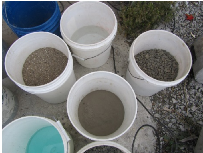
Figure 4-1: Measured Concrete Constituents Before Mixing
