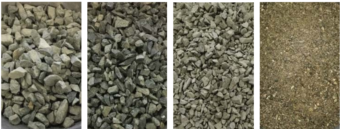
Figure 3-3: Source 2 Aggregates. From Left to Right: 3/4" Coarse Aggregate, 1/2" Coarse Aggregate, 3/8" Coarse Aggregate, Fine Aggregate
