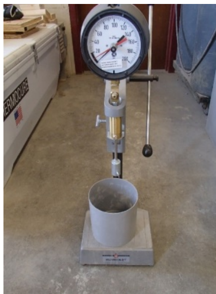
Figure 4-10: Acme Penetrometer Used to Measure Initial and Final Set Time of Concrete Mixtures & Various Penetrometer Needle Sizes
