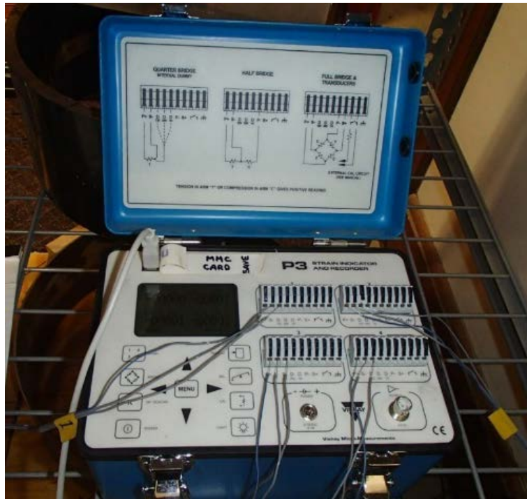
Figure 4-17: Micro Measurements P3 Strain Indicator and Recorder, Version 2.11 Used to Record Strains During the Shrinkage Test
