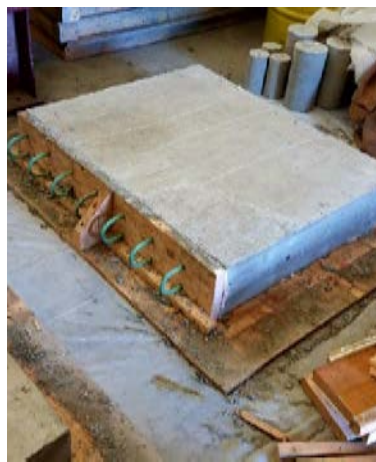
Figure 6-5: Panel Fabrication: (a) Formwork and Reinforcement; (b) Casting; (c) Cured Panels
