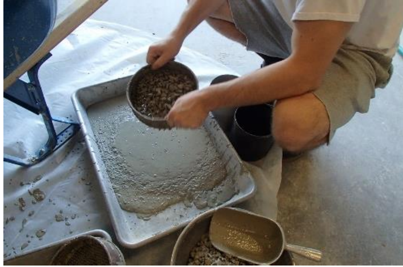
Figure 4-11: Sieving Coarse Aggregates out of Concrete to Form Mortar for Set Time Test
