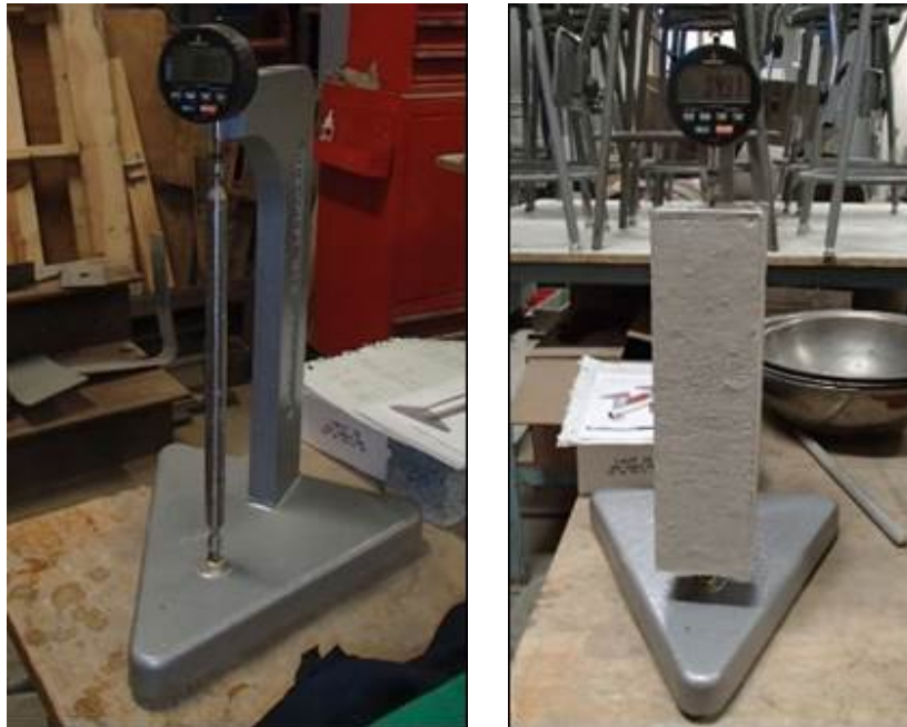
Figure 4-24: Length Comparator Shown Being Zeroed on Left and Taking a Reading of an ASR Specimen on Right
