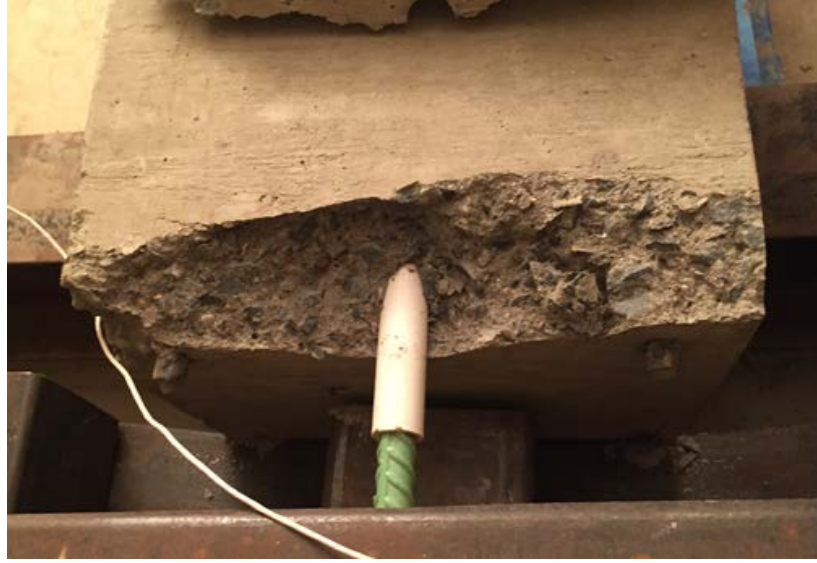
Figure 5-15: Concrete Cracking of Test Specimen 15-HD-6
