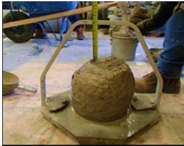
Figure 4-8: Measuring the Slump of a Concrete Mixture
