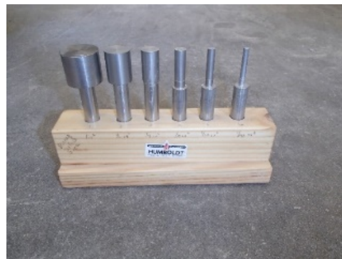
Figure 4-10: Acme Penetrometer Used to Measure Initial and Final Set Time of Concrete Mixtures & Various Penetrometer Needle Sizes
