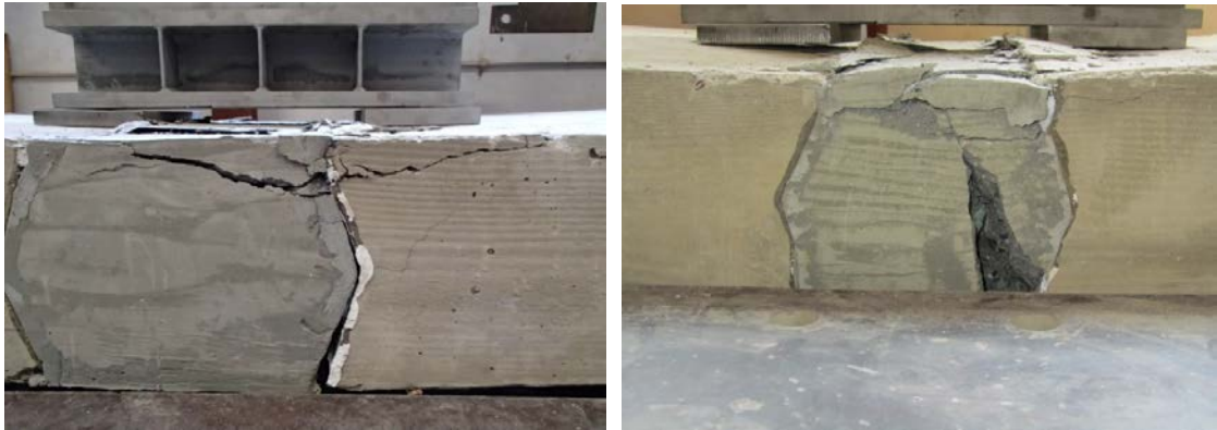
Figure 6-15: Detail View (Front) of the Joint after Failure: Specimen 1 (left); Specimen 2 (right)
