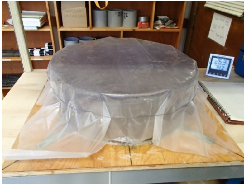
Figure 4-16: Wet Curing of the Top Surface of the Shrinkage Rings using Prewitted Burlap and Plastic Covering
