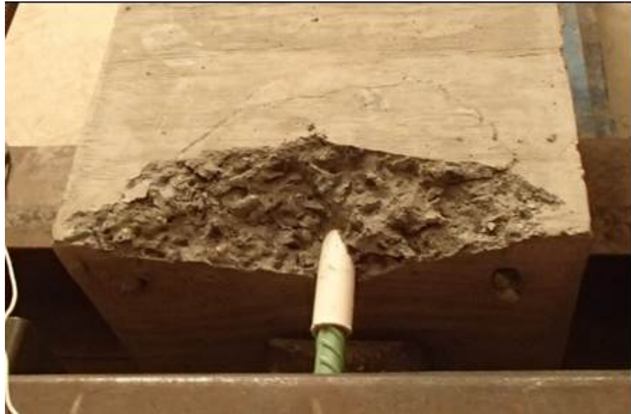
Figure 5-14: Concrete Cracking of Test Specimen 6-HD-6
