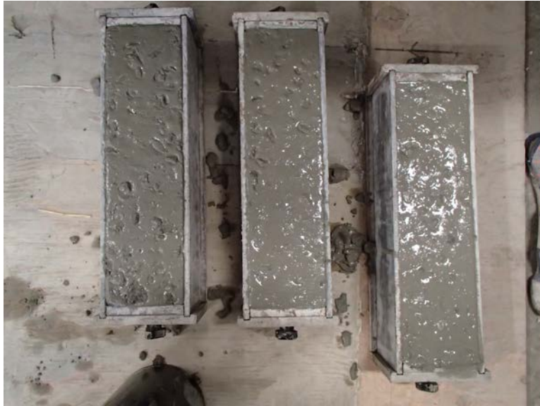
Figure 4-25: Prisms used for Freeze-Thaw Testing
