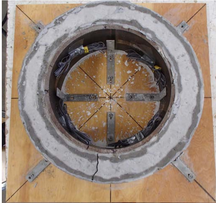
Figure 5-19: Shrinkage Cracking Occurring as One Crack in a Confined Shrinkage Ring
