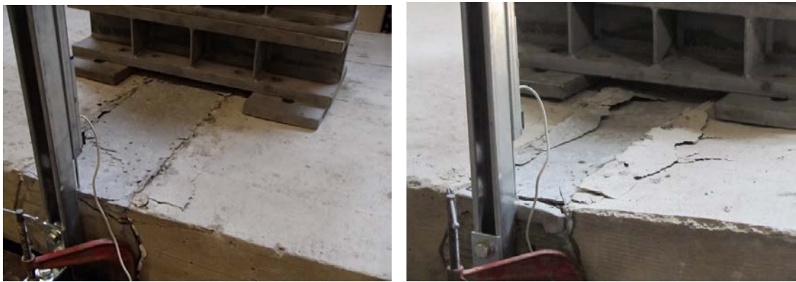
Figure 6-13: Concrete Crushing: Specimen 1 (left); Specimen 2 (right)
