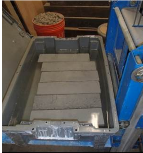
Figure 4-22: ASR Specimens Submerged in Sodium Hydroxide Solution
