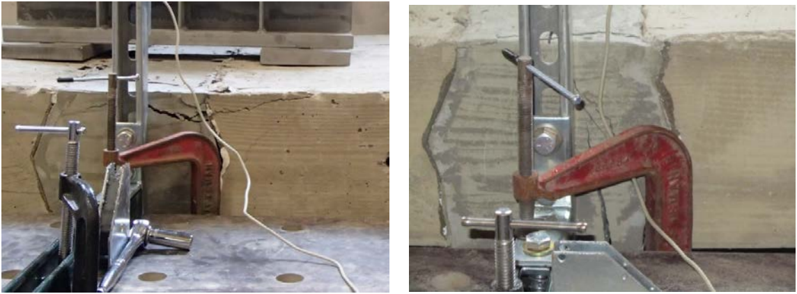
Figure 6-11: Hairline Flexural Cracks in the Panels: Specimen 1 (left); Specimen 2 (right)
