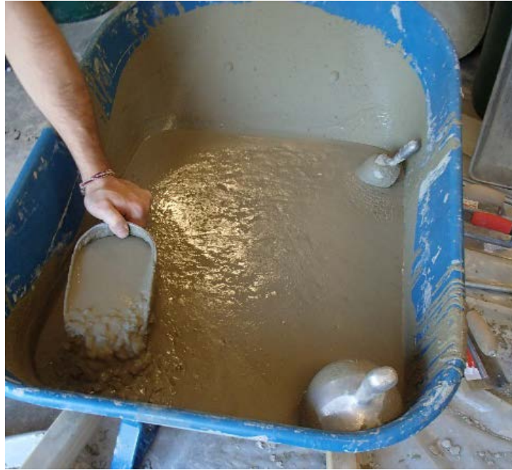
Figure 3-14: MIX 11 in Wheelbarrow Showing Segregation with Thin Paste on Top and Aggregates Being Scooped up from the Bottom
