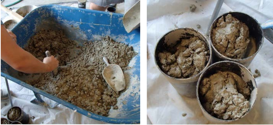
Figure 3-13: MIX 1 Thick Consistency Shown in Wheelbarrow and in Compression Strength Molds
