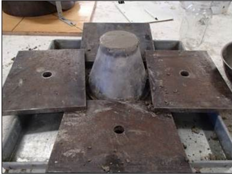
Figure 4-5: Slump Test Setup Performed on the Small-Scale Trial Batches for the HRWR Dosage Analysis
