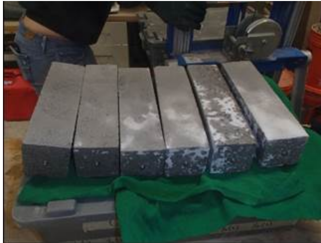
Figure 4-23: ASR Specimens Drying on Rags before Taking Length Change Measurements
