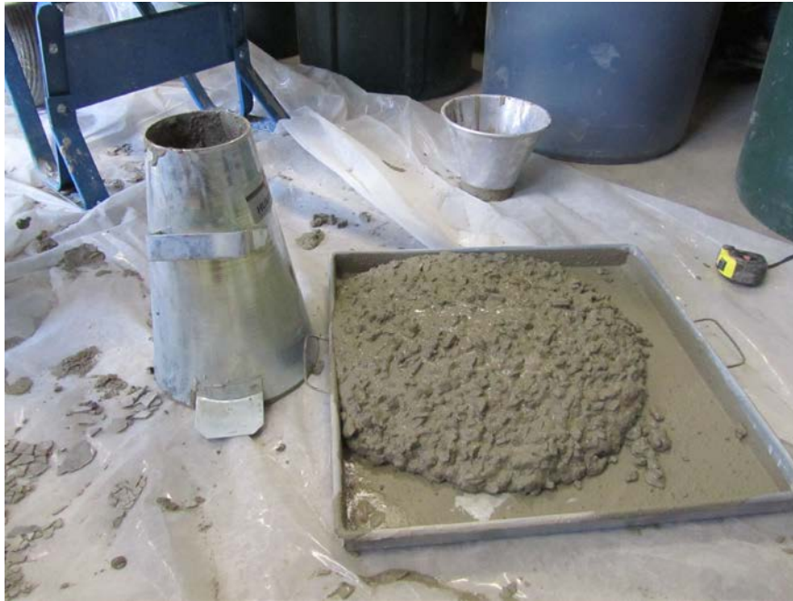
Figure 3-15: Concrete Mix with Acceptable Consistency
