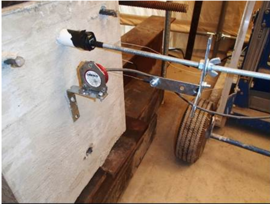
Figure 4-29: Apparatus Used for Measuring Slip During Bar Pullout Test
