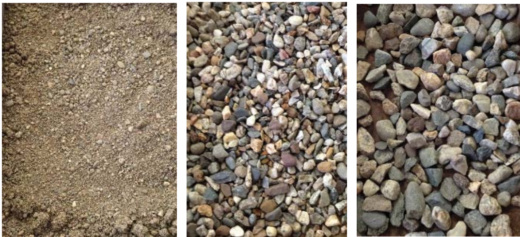
Figure 3-2: Source 1 Aggregates. From Left to Right: 3/4" Coarse Aggregate, 1/2" Coarse Aggregate, Fine Aggregate
