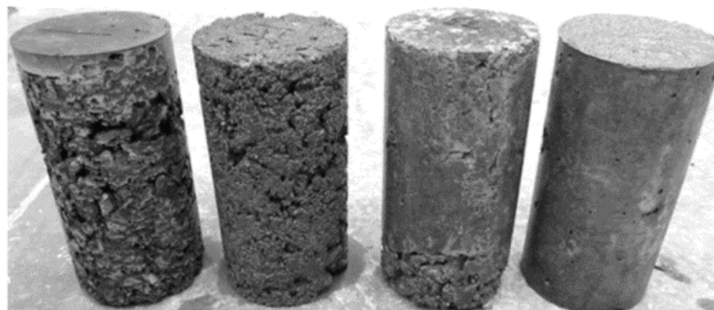
Figure 2-7: Cylinders of Concrete Made with Increasing Paste Volume from Left to Right (Taylor et al. 2015)
