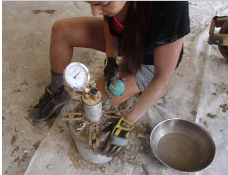
Figure 4-13: Water Injected Through Petcock of Type-B Meter for Air Content Test
