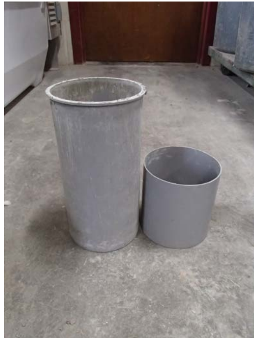
Figure 4-12: Plastic Cylindrical Mold Cut to be used for Set Time Penetrometer Tests
