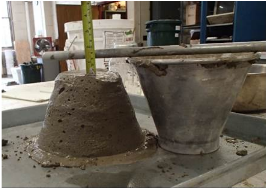
Figure 4-5: Slump Test Setup Performed on the Small-Scale Trial Batches for the HRWR Dosage Analysis
