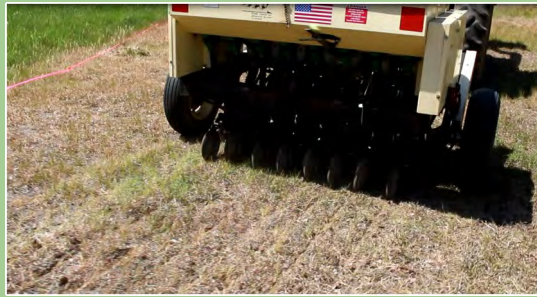
Disk coulters blades cut furrows through vegetation residue.
