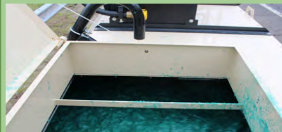
Mechanical paddle agitated hydroseeding equipment used with wood mulch.
