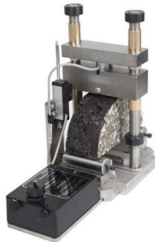
Figure 7: InstroTek's SMART SCB Jig
